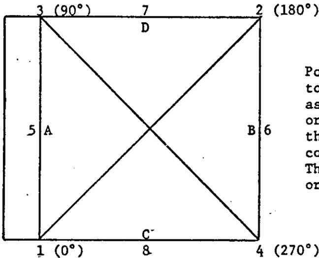
Positions of all points are referenced to the principal point of autocollimator as origin. The diagram indicates the orientation of the reference points when the camera is viewed from the back, or a contact positive with the emulsion up. The direction-of-flight fiducial marker or data strip is to the left.
