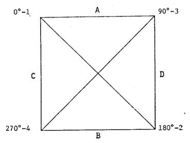
The diagram indicates the orientation of the reference points when the camera is viewed from the back. The direction of flight fiducial marker or data strip is at the top.
